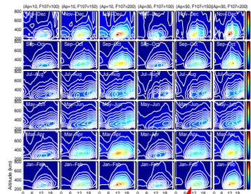
Contour plots of the model Ne in the time and height plane for 6 sets of solar and magnetic activity indices: (Ap, F107); the model Ne is computed for each bin grid with our model coefficients. (Ap, F107) values are changed for frames from left to right, and the grid value of the day number (month) is changed for frames from bottom to top. Ne scaled with color bars is in unit of  $10^{12} \text{ m}^{-3}$ .
